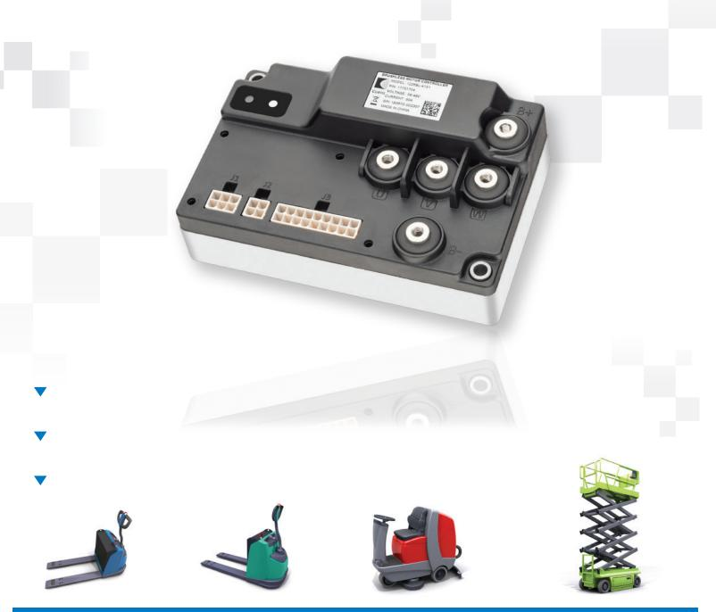
The Curtis Model 1226BL Motor Speed Controllers provide efficient, optimal control of Brushless DC drive motors for battery powered vehicles. Optimized for use on light duty Class III pallet trucks and sweeper scrubber floorcare machines. Highly flexible programmability allows them to be applied on any low power BLDC motor application.
